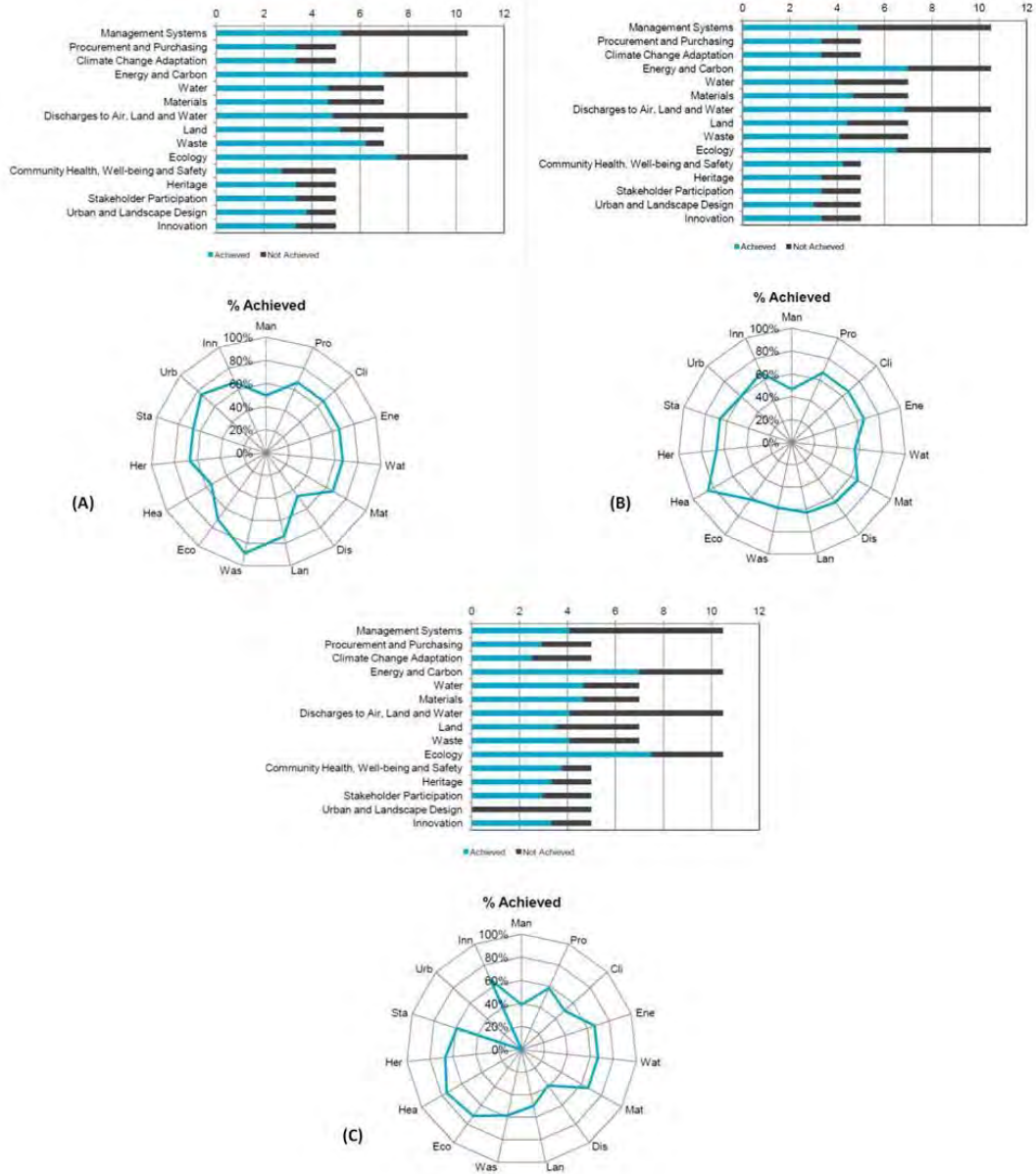
Figure 6. EastLink Transportation Corridor Design and Delivery Phases Rating using IS Tool: (A) Design, (B) As Built, and (C) Operation
