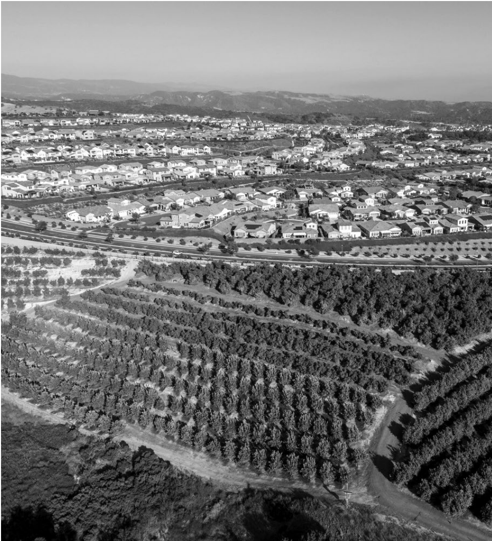
The Rancho Mission Viejo Esencia community is surrounded by an irrigated buffer of citrus trees to reduce potential wildfire exposure. Photo: David Lloyd, SWA
