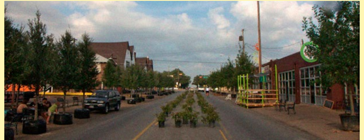
A three-lane street was transformed to two lanes by a planted median, street trees and a shared seating area.
